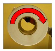
9. Install the stopper disc onto the spindle and slide into place. The stopper should be positioned to prevent the roll from moving too much from side to side but be allowed to spin freely.
