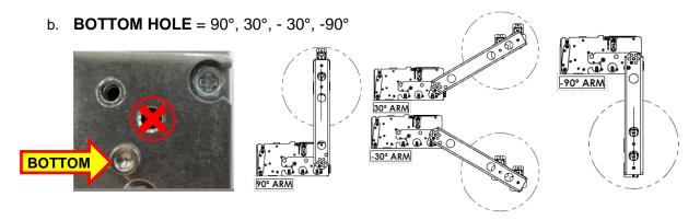
4. Install the roll holder arm onto the mounting plate and secure it in place with the provided ¼" Hex head #8 Taptite screw. Below photo shows the arm set to the 30° positions. Arm position will vary depending on what degree position is used.
