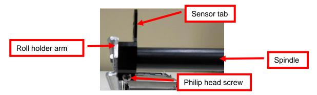
b. For 58mm, the block should be spaced 0.474" away from the roll holder arm. The roll needs to line up with the center infeed guide. See below photos.
