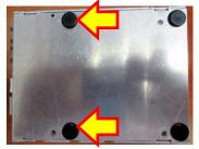
7. Install the floor plate onto the bottom of the Lemur-X UPG printer. Align the two holes on the floor plate up with the two mounting holes on the printer. Install the two 3/16" hex head Taptite screws and tighten.
