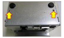
8. Flip both the Lemur -X and attached floor plate so all rubber feet are facing down.
