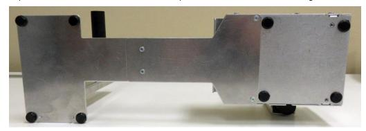
9. Align the two holes on the roll holder up with the two mounting holes on the floor plate. Install the two 3/16" hex head Taptite screws and tighten.
