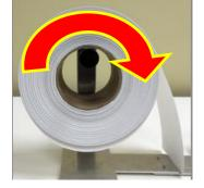
12. Install the adjustable stopper disc onto the spindle and slide into place. The stopper should not be binding against the roll to prevent it from moving freely.
