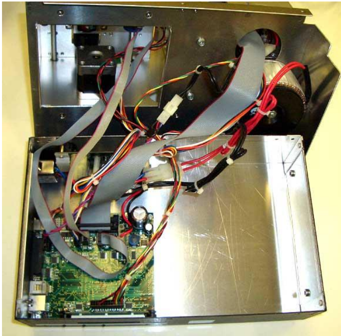
Above photo shows lower electrical box with access cover removed
