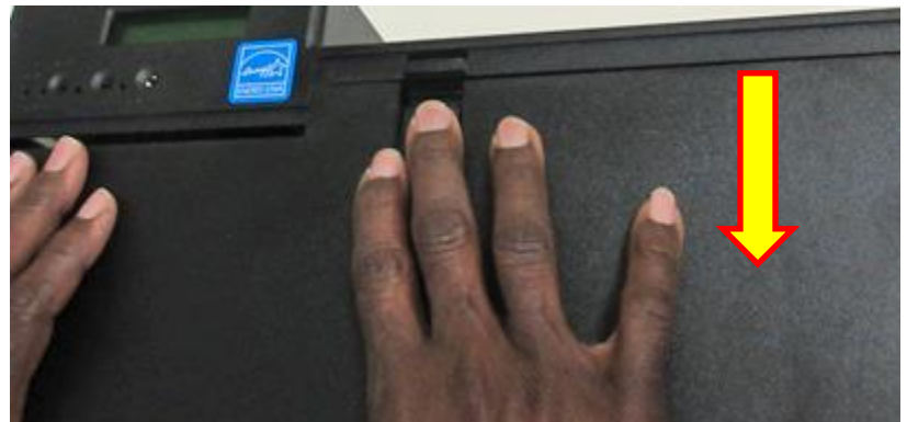
Press down on the locking tab to unlock and slid cover back a little.
