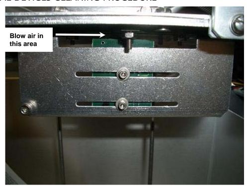
There is one opto devices mounted on a silver aluminum bracket beneath the paper guide. The opto controls ticket cut/tear position. Over a period of time there may be an accumulation of ticket dust on the opto eyes themselves. This paper dust could cause erratic operation of the printer.
