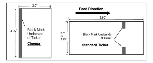
When loading 5.50" long ticket stock the black timing mark should be closest to the leading edge of the ticket (the first part that goes into the printer). When loading 2.0" long cinema ticket stock the black timing mark should be furthest away from to the leading edge of the ticket (the first part that goes into the printer).
