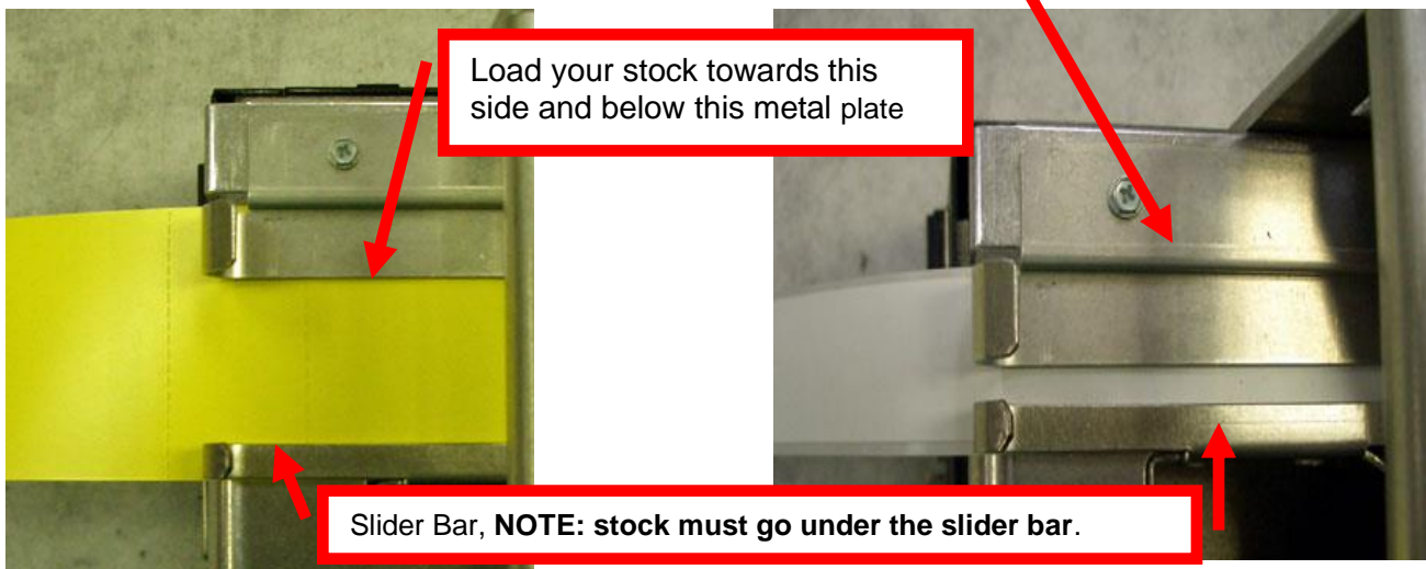
Above photo is of ADJ2 set for 2" wide stock Above photo is of ADJ2 set for 1" wristband stock
