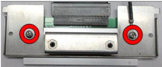
2. Gently unplug the cable from the old print head and plug it into the new print head. The cables are keyed (see examples below). The keyed position must be lined up while plugging the cable into the print head. **You should not have to use excessive force to do this.**
