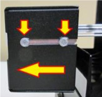
3. Remove the two 3/16" hex head screws that hold the upper paper guide upper rail in place.
