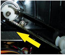
15. Install the cutter assembly back onto the print cage and make sure the ground wire is attached back on as shown in step #4.
