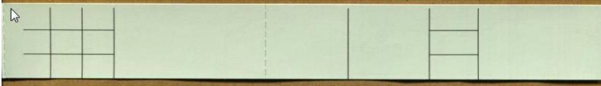
13. Click on the FAA Test Tickets button and go to the FAA2016 folder found in the firmware directory. Send the FAA\_Tower20.txt file to the printer. Twenty tickets will printout. The cut position and text alignment should be similar on all tickets. Attach one ticket to the check sheet.
