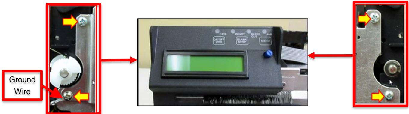
5. The electronics cover may be gently lifted up a little to enable the cutter assembly to separate from the print cage. This will enable you to get access to the platen.
