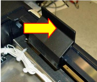
4. Flip the head back toward the rear of the printer. Denote what slot the print head was taken out of.
