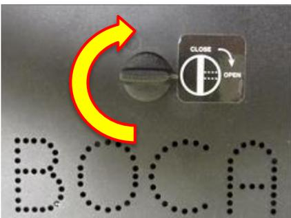
To install the cover back in place, make sure the knob is in the unlocked position. Fit the cover onto the opto of the printer and turn the knob to the locked position.
