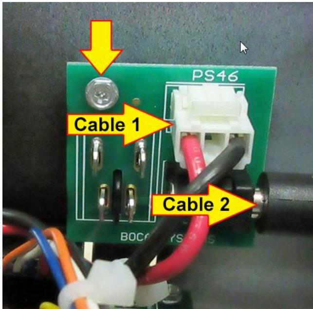
4. Install the replacement switch power board by reversing the above steps.
