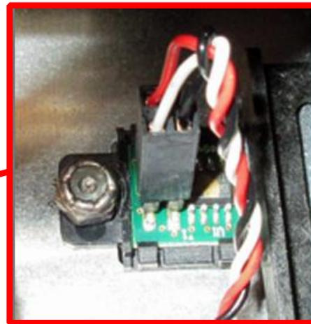
4. Remove the 1/4" nut with either a nut driver or socket.
