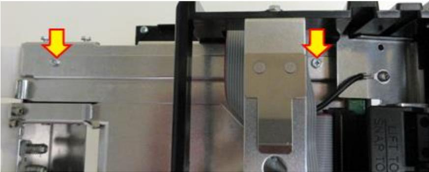
4. Remove the Phillips head screw that holds the cut opto onto the mounting bracket. Unplug the connector from the opto.
