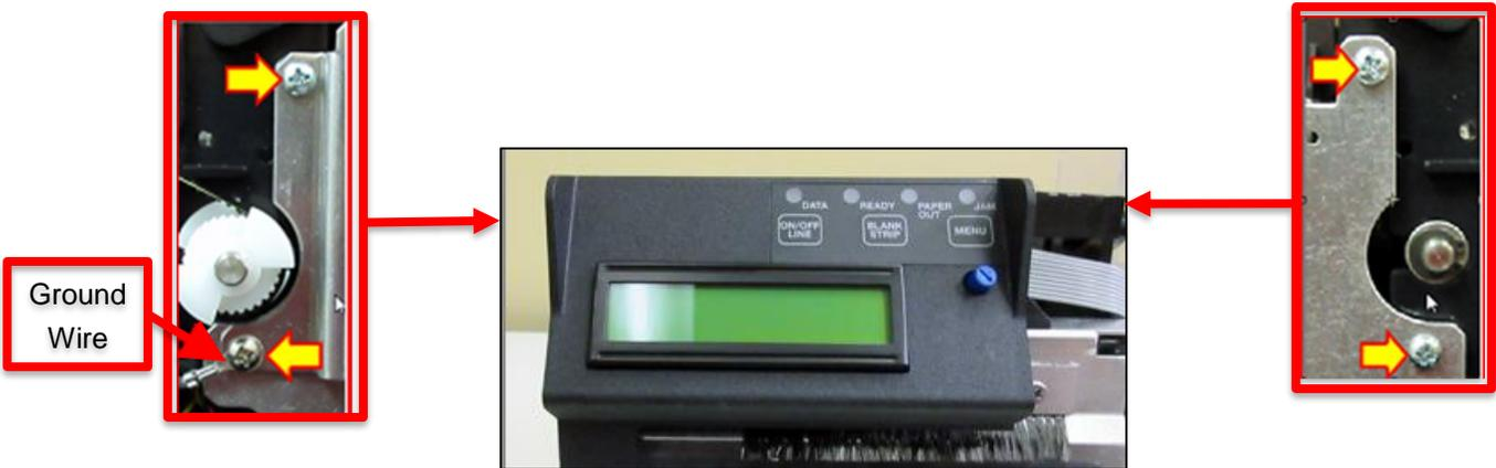
4. Remove the one 3/16" hex head screw that is holding the control panel onto the cutter. Place control panel out of the way.
