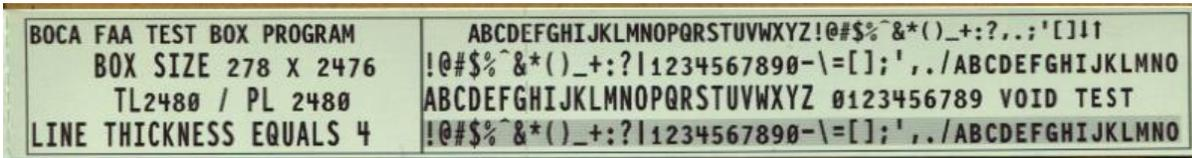
14. With the printer offline. Pressing the ON/OFF LINE & BLANK STRIP buttons simultaneously will cause the below printout. Attach sample to test sheet.
