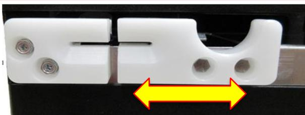
Slider may be adjusted for different width flight strip stock.
