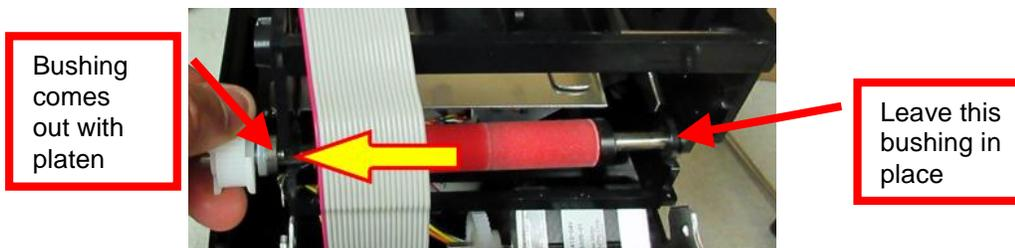
10. Install the new replacement platen in place. Install the grip ring back onto the shaft.
