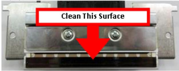
7. Install the head mounting plate by reversing the above procedures. Make sure the print head mounting plate tabs are in the back slot of the print cage slots.
